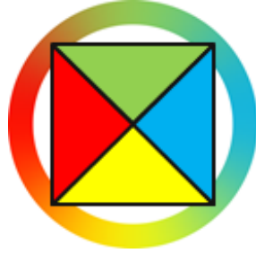
Figure 5.5: A 2D anisotropic voxel with per-face color values. Image courtesy of [Mit12].
